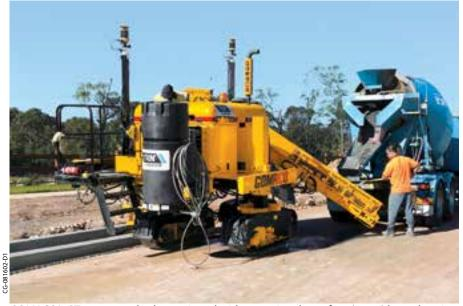
GOMACO's GT-3200 can also be equipped with an optional 13.5 foot (4.1 m) long charging conveyor to move concrete to the hopper.
