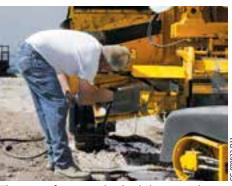
The auger features a latched clean-out door at the receiving end of the hopper.
