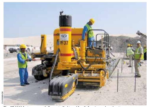
The GT-3200 features smooth G+ controlled travel for slipforming curb and gutter.
