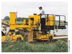
The GT-3200 slipforms a walking trail with an undermounted mold.
