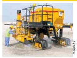
A high-pressure or low-pressure water system is available for easy cleanup.
