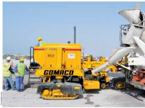
The operator's platform provides an ample view of the entire slipforming operation.
