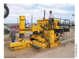
The operator has an excellent view of both the trimmerhead and mold when using the simultaneous trim/pour concept.
