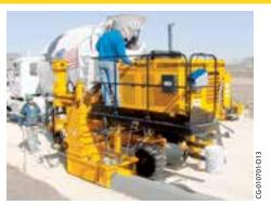
The GT-3200 can be equipped with three pneumatic tires.
