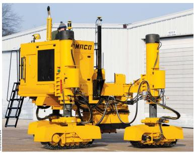
The Xtreme GT-3600's tracks can rotate farther than ever before. The rotary-sensored slew drives allow the tracks to rotate 90 degrees and more for quick side travel and to slipform a tight radius.
