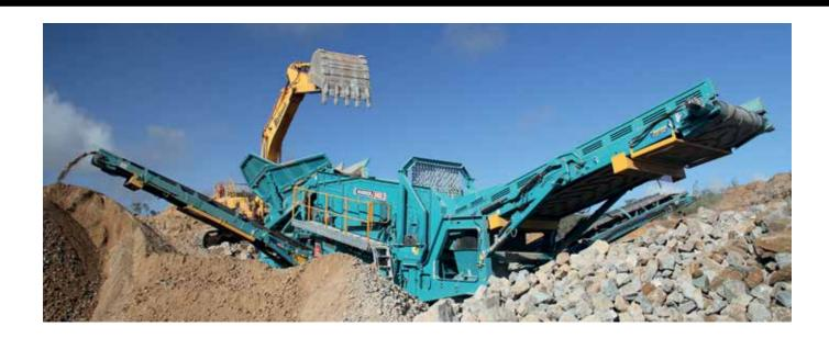
Specially designed for large scale operators in the quarrying and mining sectors, the new Powerscreen® Warrior 2400 is capable of handling larger feed sizes and throughputs. It features a heavy duty incline screen with a high amplitude triple shaft drive mechanism, lending it to screening, scalping, 2 or 3 way splitting and stockpiling materials like aggregates, topsoil, coal, construction, demolition waste and iron ore.
