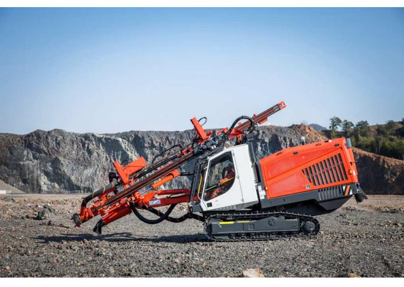
Tiger DG800 is a hydraulic, self-propelled, selfcontained, crawler based surface drilling rig equipped with a cabin (F.O.P.S. and R.O.P.S.) and rod handling system.
