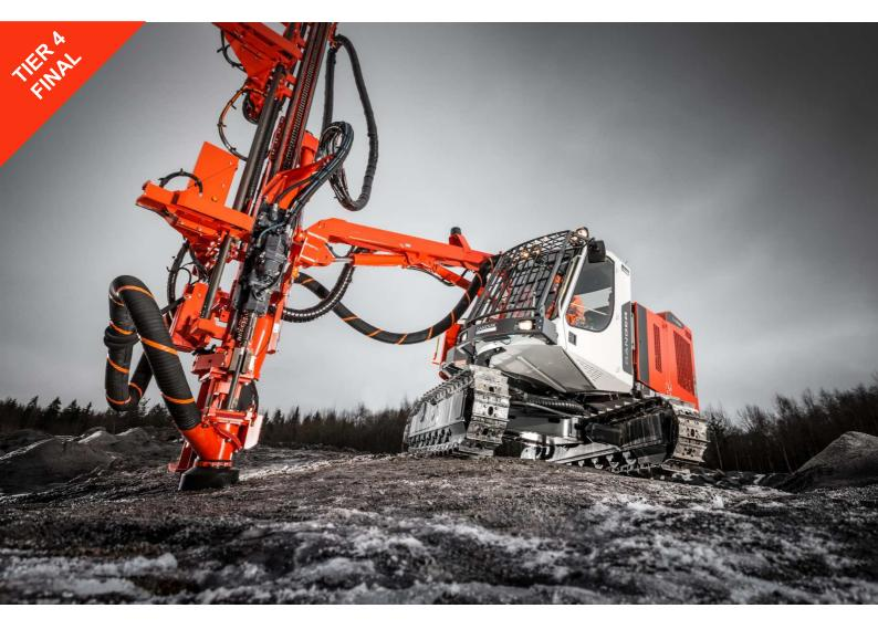
Ranger DX600 is a hydraulic, self-propelled, self-contained, crawler based surface drilling rig equipped with a cabin (F.O.P.S. and R.O.P.S.) and rod handling system.
