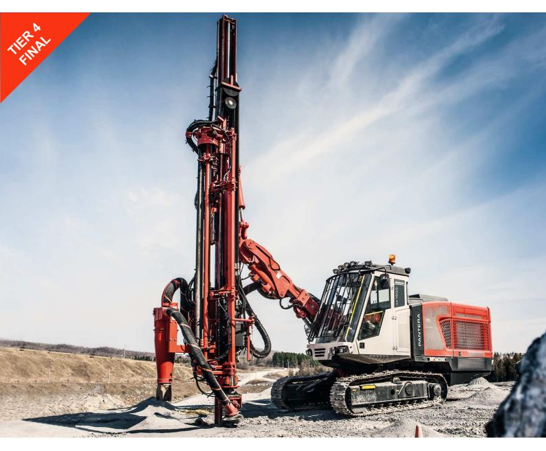
Sandvik Pantera DP1500i is intelligent, self-propelled, self-contained, crawler based surface drilling rig equipped with a cabin and a rod changer.
