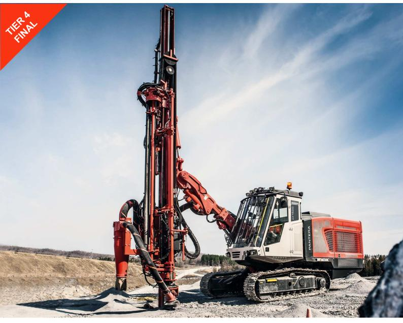
Sandvik Pantera DP1100i is intelligent, selfpropelled, self-contained, crawler based surface drilling rig equipped with a cabin and a rod changer.
