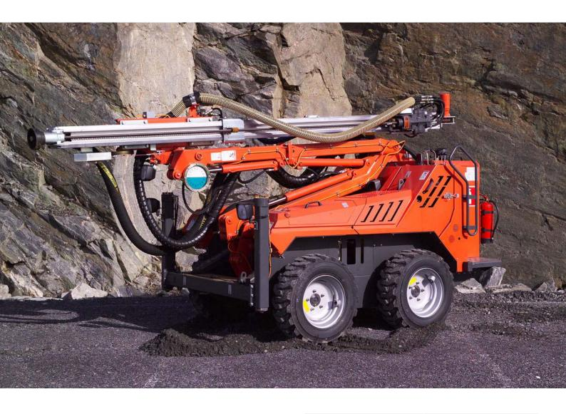
Sandvik DC121R is a remote controlled, hydraulic and self-propelled drilling unit on a 4-wheel drive carrier.
