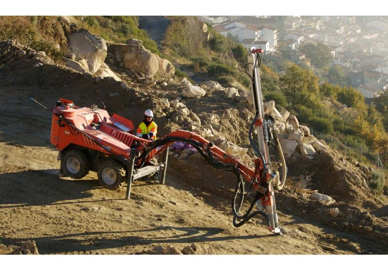
Sandvik DC120 is a hydraulic, self-propelled drilling unit on a 4-wheel drive carrier.
