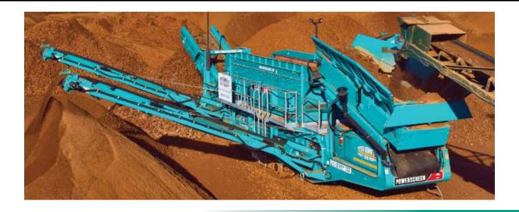
The Powerscreen<sup>®</sup> H range features horizontal screens ideal for handling high volumes of sticky materials and for the exact, fine sizing demanded in many construction contracts. The H6203 & H6203R offer higher capacity output; up to 800tph compared with up to 600tph with the H5163 & H5163R models.
