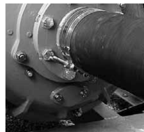
Pump drain for cold climate applications
