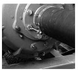
Pump drain for cold climate applications
