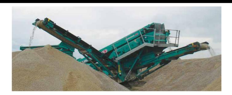
The Powerscreen® Chieftain 1400 is one of Powerscreen's most popular screening products and is ideally suited for small to medium sized operators and contractors who require a versatile product capable of operating in a number of applications such as sand and gravel, aggregates and recycling. User benefits include hydraulic folding conveyors for a quick set-up time, screen walkways and access ladders for ease of maintenance, and a drop down tail conveyor to aid screen media changes.
