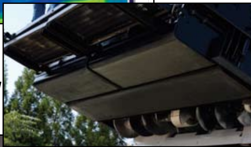
Heat is distributed evenly across the plate after only 30 minutes of heating. The heating elements are heavy-duty and only need to run at 1/3 rated capacity to keep the screed hot.
