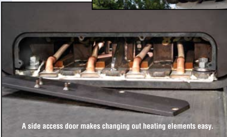
Heat is distributed evenly across the plate after only 30 minutes of heating. The heating elements are heavy-duty and only need to run at 1/3 rated capacity to keep the screed hot.
