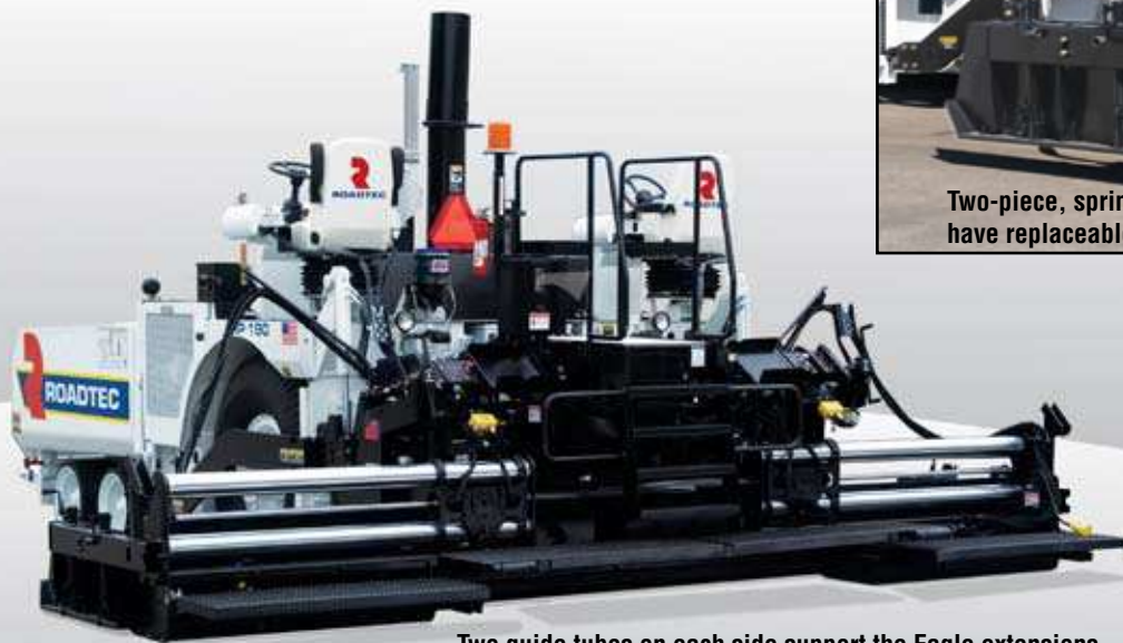
Two guide tubes on each side support the Eagle extensions.
