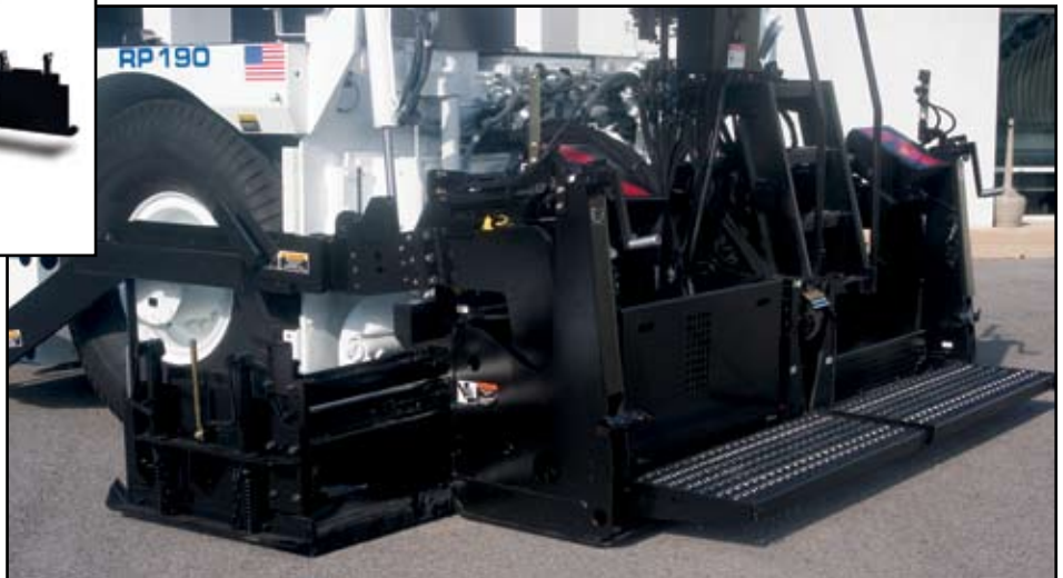
Top: Front view of SC screed with extension retracted. Right: Rear view of SC screed with extensions out.
