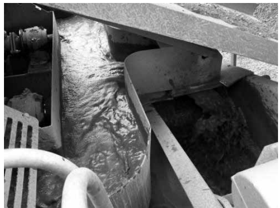
Flume system for transfer from hull to screen
