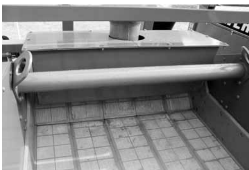
Modular screen decks and side protection liners
