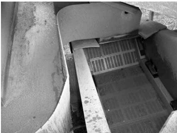
Sloped back panel and modular screen decks
