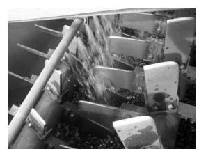
Spiral design axles with high tensile and quickly replaceable blades
