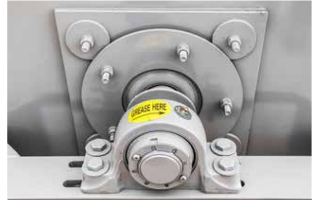
SLINGER PROTECTS LOWER BEARING
