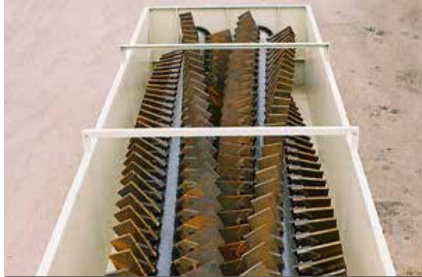
SPIRAL PADDLES FOR CONTINUOUS AGITATION
