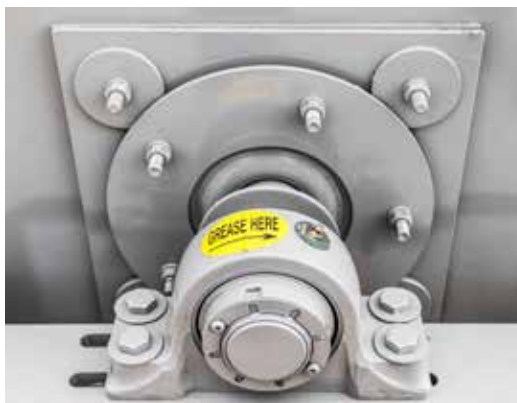
SLINGER PROTECTS LOWER BEARING
