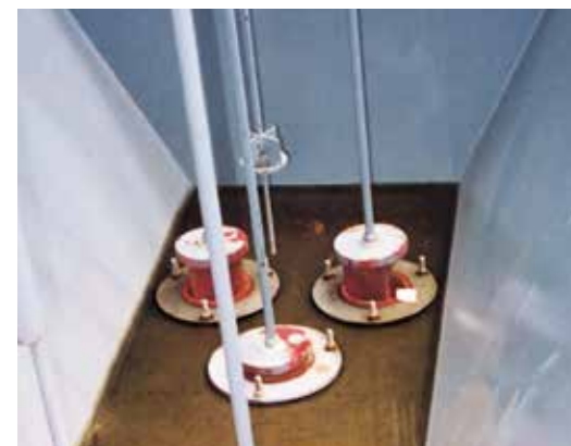
URETHANE DISCHARGE VALVES
