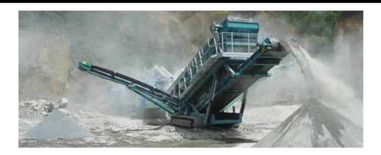
The Powerscreen® Chieftain 2400 is the largest mobile screen in the range aimed at mining, quarrying and recycling operators who require high volumes of finished sand, gravel, coal and crushed stone. The Chieftain 2400 features a hopper suited to direct feeding from a crusher, an oversized heavy duty screen unit and a 4th auxiliary conveyor for recirculating material for secondary reduction and re-screening.
