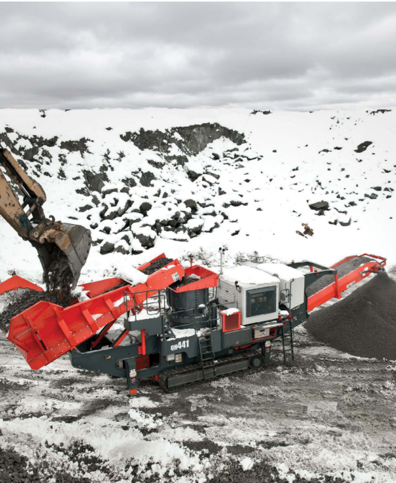
Featuring the proven, high performing Sandvik CH440 Hydrocone.
